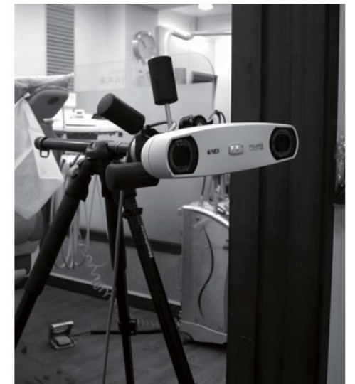
Fig 2. Optical tracker (Polaris Vicra System, Northern Digital, Waterloo, Canada).
